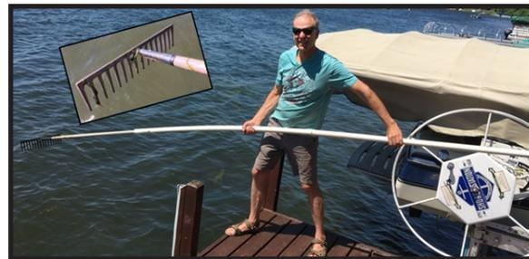
Attach a rake head to a 10' length of a 1¼" diameter PVC pipe to make your own weed rake.
